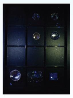
Only the natural diamond on the bottom right shows some blue fluorescence. Simulants and lab grown diamond will never show fluorescence under Long UV illumination.
