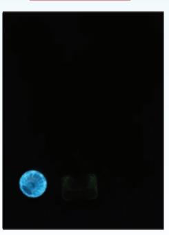
These HPHT and CVD lab grown stones show phosphorescence. Simulants and natural diamonds show NO phosphorescence whatsoever.
