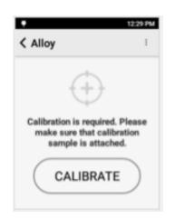
Place the 316 coupon that came with the unit on the nose. If the coupon is not available, use a clean, known 316 steel sample. Make sure the 316 coupon completely covers the analysis window. Tap "CALIBRATE" to begin the process.
