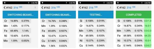
Tests report findings in real time, so as the test continues and more information is obtained, the data on the screen will be updated. When the "COMPLETED" screen appears, the test is done and the final values are given.
