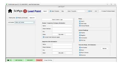
From this screen, you can select what results you wish to view by filtering by date or job number on the left side. The middle of the screen is information on who performed the work and the inspection site. The right side allows the user to select the information they would like displayed.
